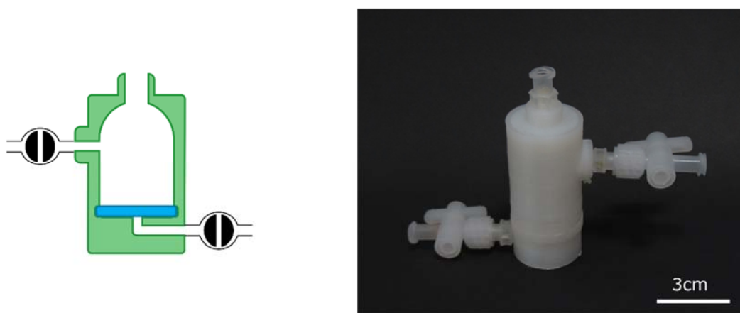
Fig. S20: Schematic diagram (left) and photograph (right) of filtration module used to achieve the synthesis of lamotrigine.
